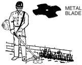
NOTE: Remove the trimmer head before installing the weed blade. To remove the trimmer head, align hole in the dust cup with the hole in the side of the gearbox by rotating the dust cup. Insert a small screwdriver into aligned holes. This will keep the shaft from turning while loosening the trimmer head. Remove the trimmer head by turning clockwise. Remove the screwdriver.
